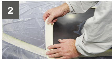
2 Apply the appropriate 3M masking products to suit the repair area and move vehicle into the booth.
