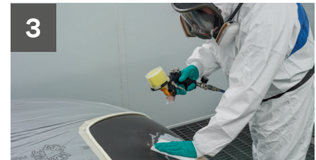
3 Blow and wipe down with a 3M™ Tack Cloth.
